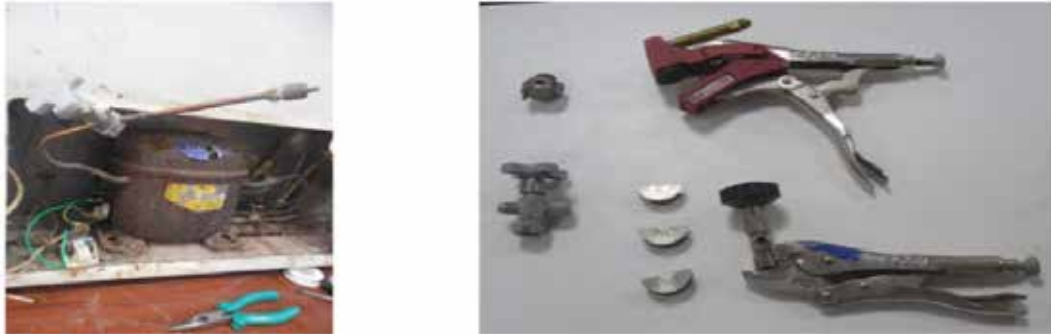
Figure A-2.1: To access the system at the filter drier when recovering refrigerant use line piercing pliers and valve.
