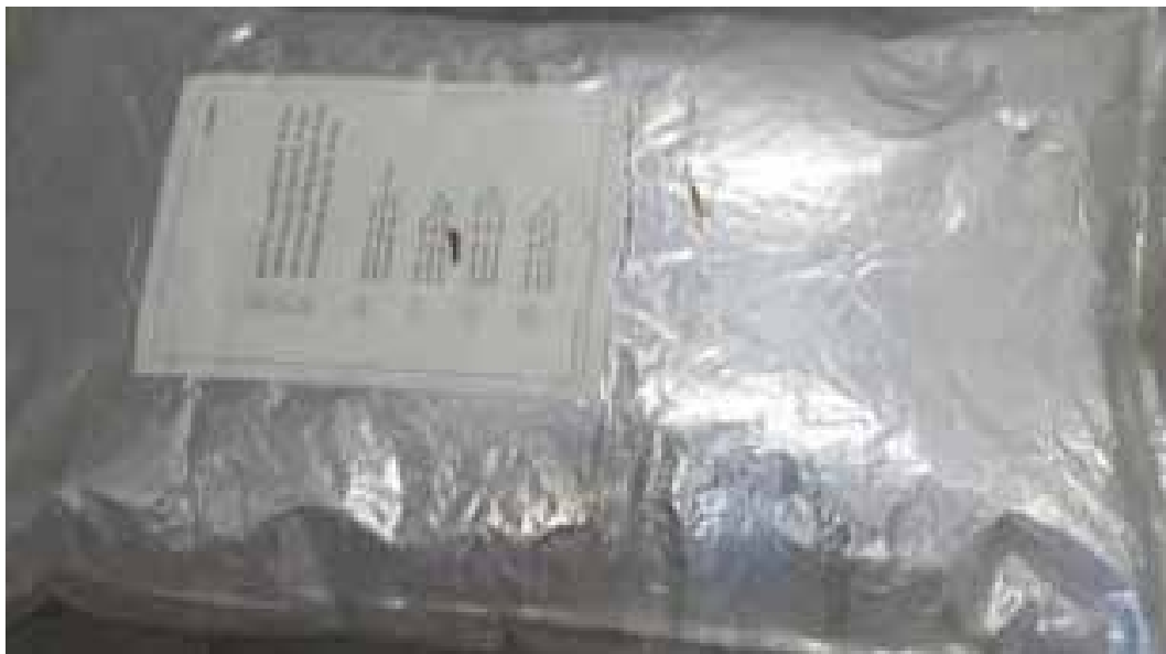
Figure A-2.3: For the recovery of refrigerant during field repairs a special bag has been designed. The inside of the bag is made of a foil resistant to the specific refrigerant. There is a layer of gas proof aluminium foil and an additional layer of foil which prevents the penetration of oxygen. The bag is equipped with a 1/4" flare connection with schrader valve This bag is used for recovery and transport of refrigerant.
